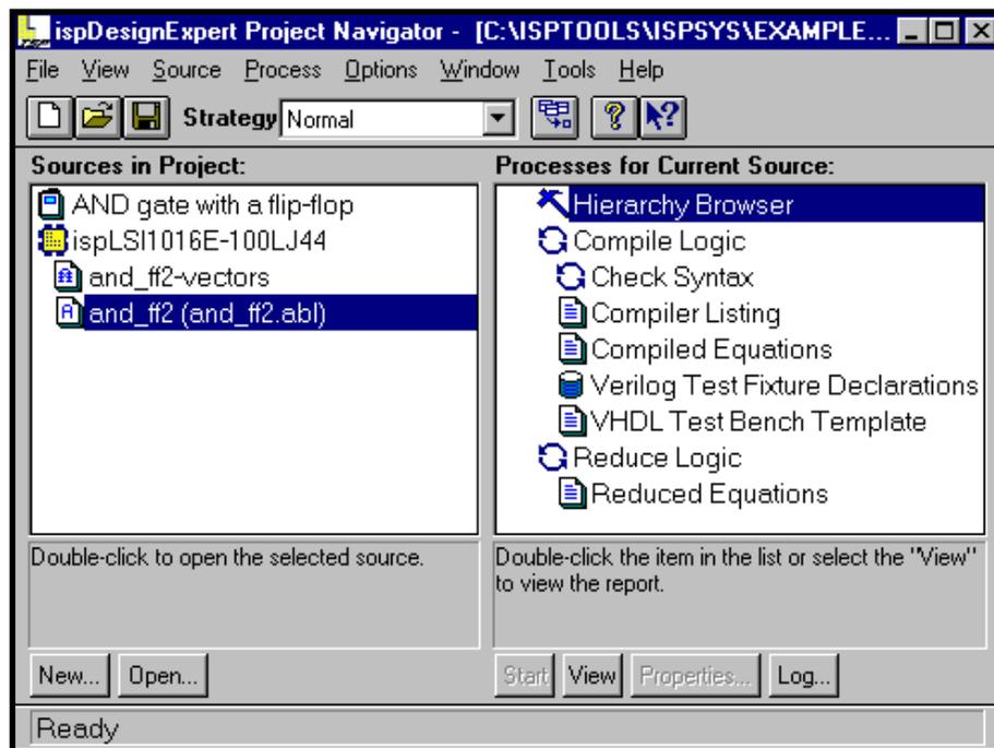
Figure 3-7. Project Navigator Window with `and_ff2.syn` Loaded
