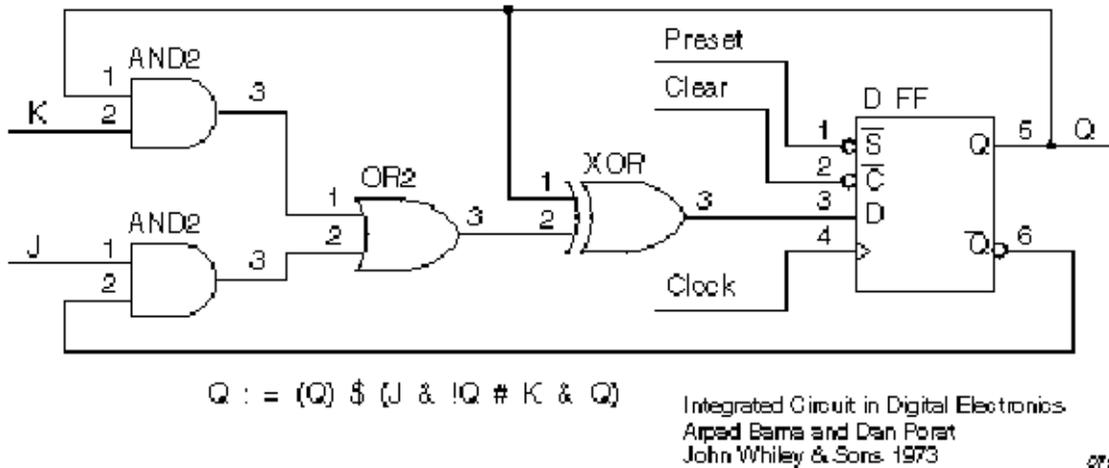
Figure 4-11. JK Flip-flop Emulation, D Flip-flop with XOR
