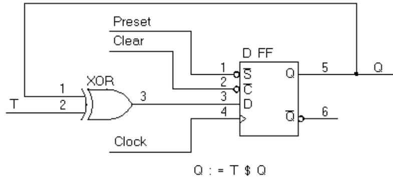
Figure 4-10. T Flip-flop Emulation Using D Flip-flop
